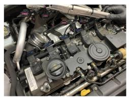
3 Remove the first 2 coil packs on the left side and then the 3 x T20 screws holding the PCV pipe to the top plate. Then pull the rubber actuator hose away from the hard pipe.
