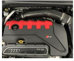
Remove the 3 x 10mm nuts from the top of the coil packs and then unclip the coil pack connector plugs. Next, unclip the cam-sensor, and once the assembly is loose you can remove the 10mm earth wire connector on the left.
