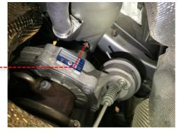
12 Raise the car again and install the other M6 captive bolt to the underside of the inlet to the turbo.
