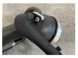
10 Install the machined inlet adapter in the inlet pipe, ensure the 0-ring is seated correctly in the adapter before installing the pipe.
